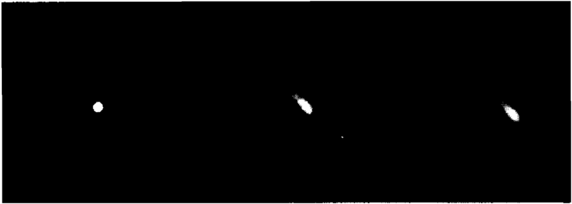
FIGURE 4.1.4 Progression of the steerable streak filter. (left) The scene image. (middle) Intermediate results after a single iteration of the filter. (right) Results from two iterations of the streak filter.
