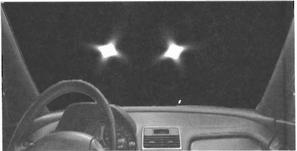
FIGURE 4.1.8 The steerable streak filter was used to streak the headlights of oncoming traffic in this image.
