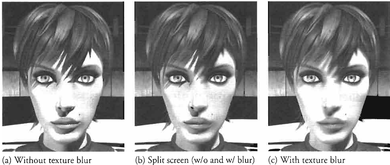
FIGURE 2.8.1 Comparison of skin rendering with and without the texture-space blur operation. Images from ATI's demo Ruby: The Double Cross. © ATI Technologies 2004.
